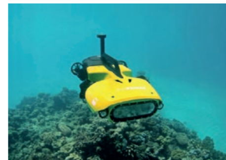
The underwater drone “RangerBot” on the lookout for coral-eating crown-of-thorns starfish. Image: Great Barrier Reef Foundation
